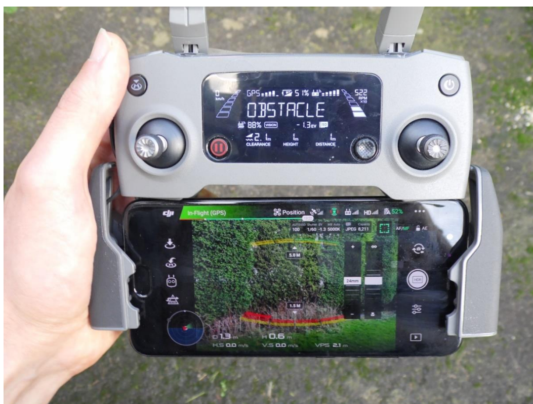
Figure 2. Drone remote-controller displaying drone camera view and flight information
