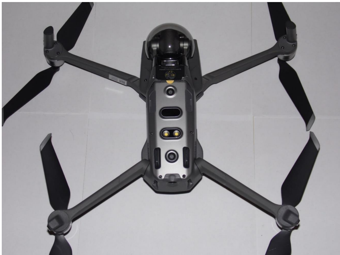
Figure 1. Ground proximity sensors on the underside of a drone
